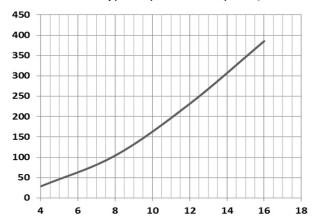
Cold Plate R<sub>th</sub>, °C/W, vs Flow Rate, liters/min
