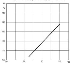
FET Tj vs Coolant inlet Temperature. Rth = .0168 K/W, lo = 200A, fsw = 15 kHz
