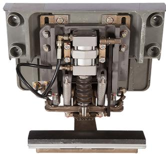
Current collector devices are used by Metro to collect the energy from the third rail to energize the Electrical Multiple Unit installed in the trailers.
