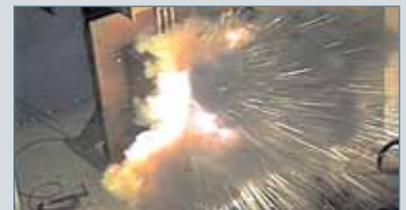
*Arc Flash in test lab. Test conditions: 250V; 15,000A; 0.1 second clearing. Incident energy was measured to be 8.5 cal/cm<sup>2</sup> at 18".*
